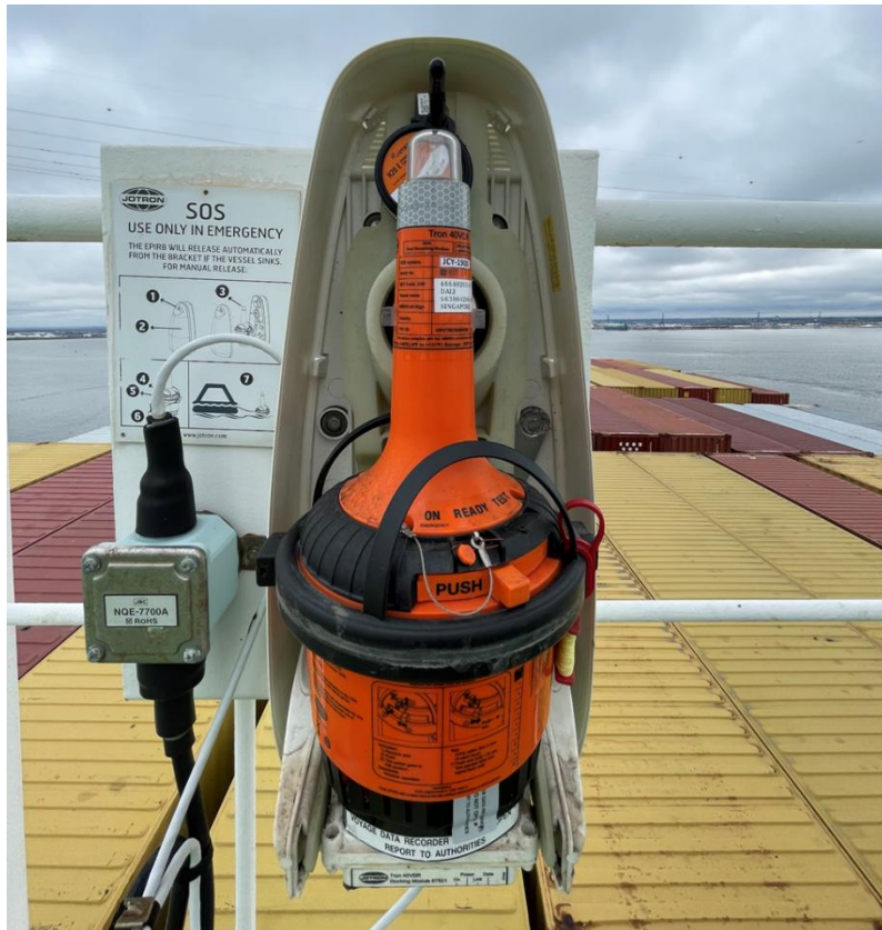
Figure 4. Photo of Tron 40VDR float free VDR capsule mounted above the wheelhouse on an exterior deck rail on the Dali .
