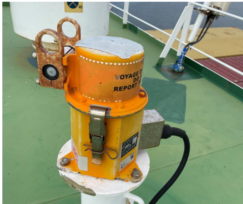
Figure 3. Photo of L3 fixed protective capsule mounted above the wheelhouse on the Dali .
