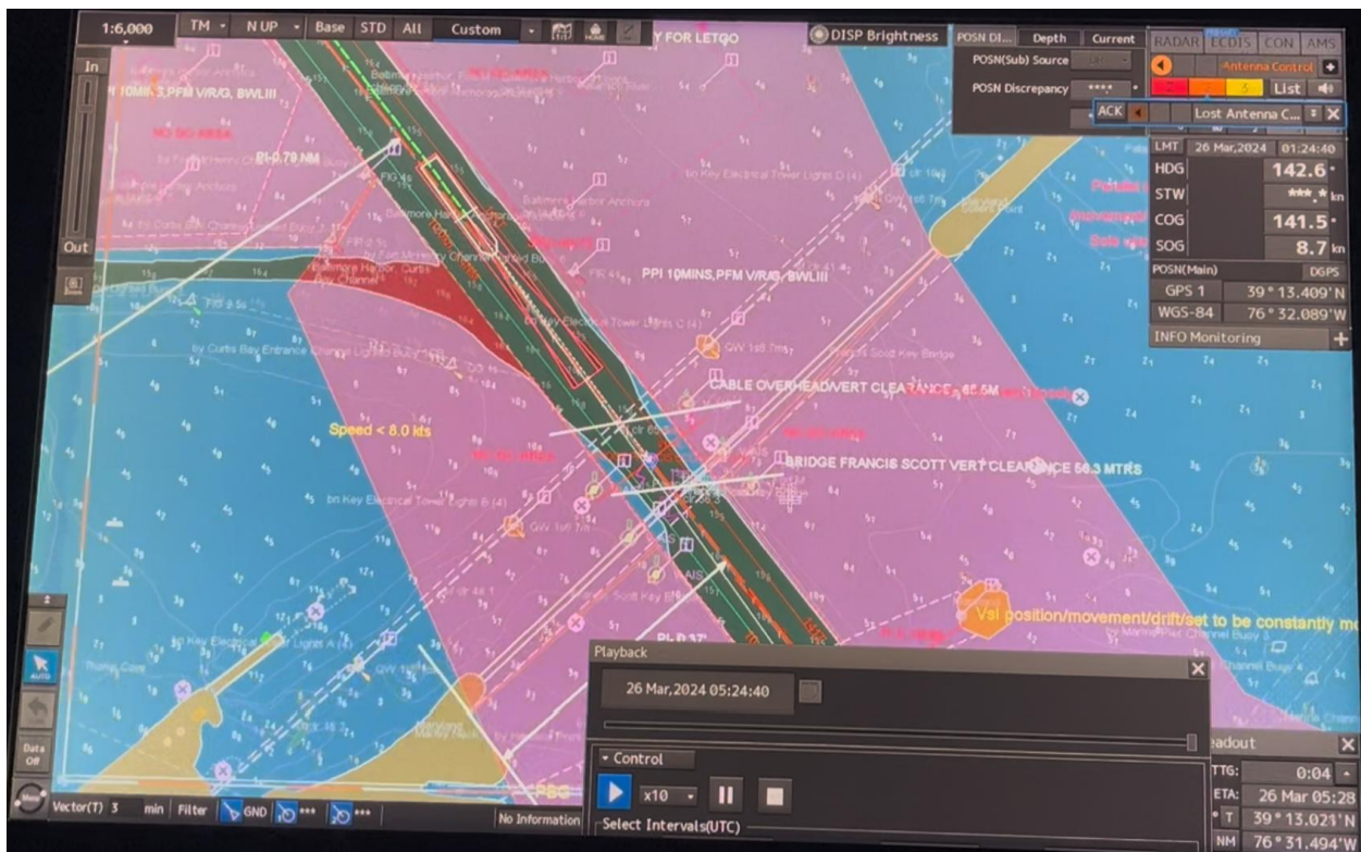
Figure 178. ECDIS playback image at approximately 01:25:41 EDT.
