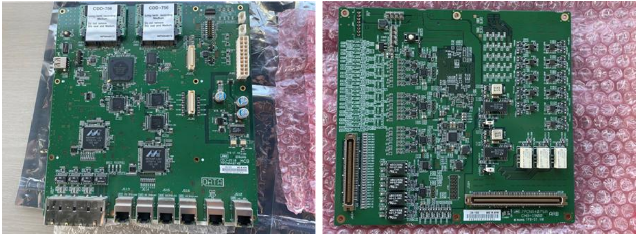
Figure 8. Photos of JCY-1900 internal memory components: main control board (see left photo) and audio recording board (see right photo).
