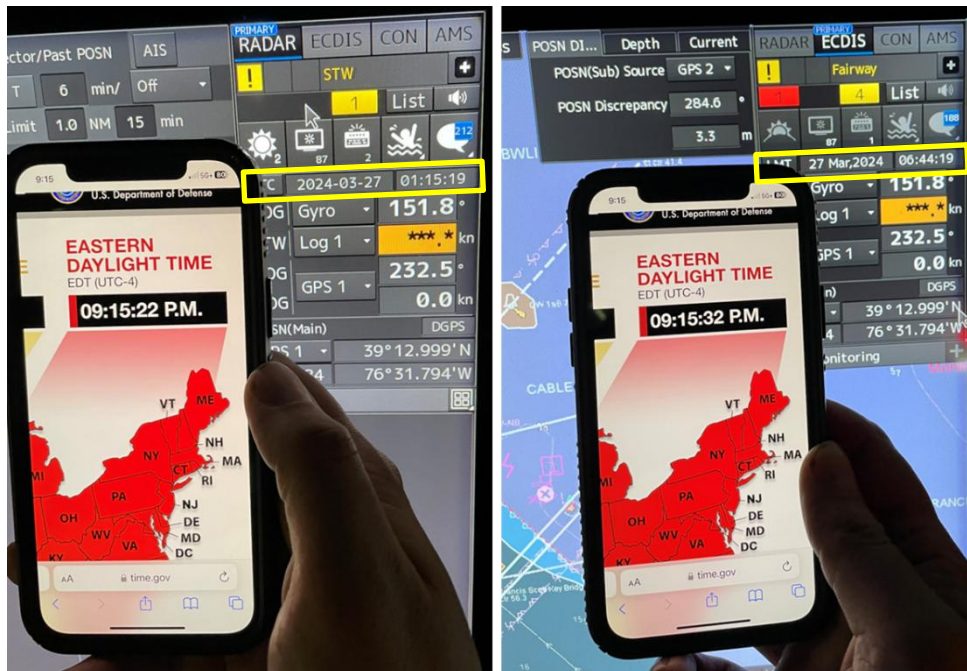
Figure 10. Photos of time sync verification on the Dali for the radar image (see left photo) and ECDIS image (see right photo) on March 26, 2024 EDT.
