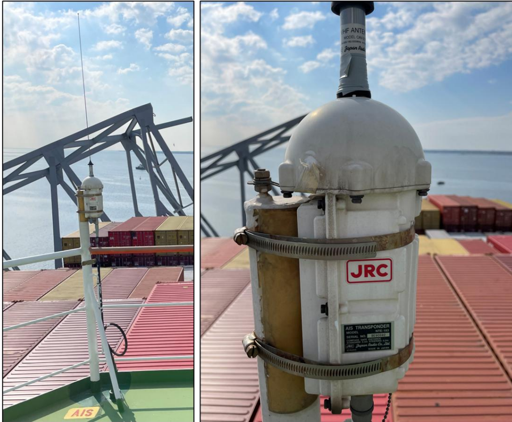
Figure 5. Photos of AIS transponder mounted above the wheelhouse on an exterior deck rail on the Dali .
