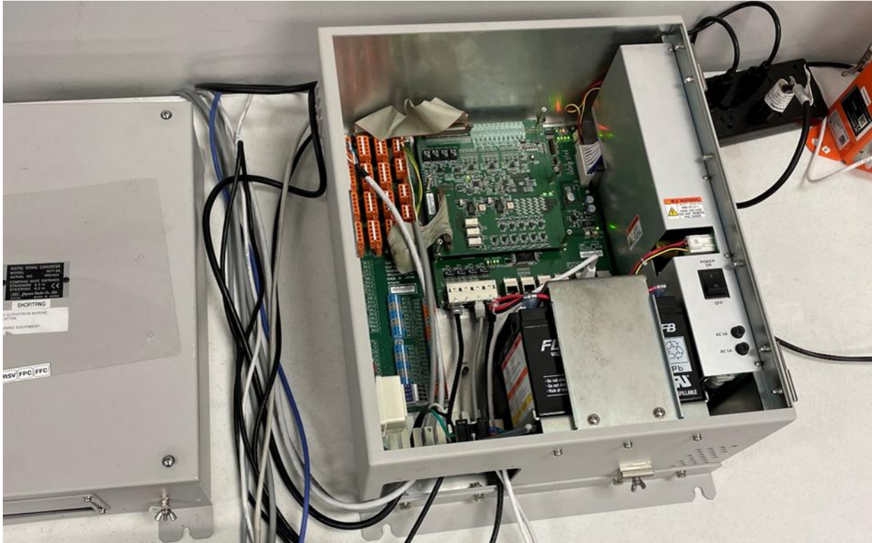
Figure 9. Photo of the internal memory components placed into a surrogate JCY-1900.
