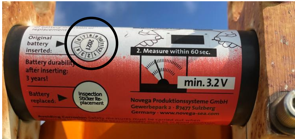
Figure 1. Photo of the VDR acoustic beacon located on the L3 fixed protective capsule mounted above the wheelhouse on the Dali . The original insertion battery date, May 2021, is circled. The acoustic beacon is listed with 3 years of durability after insertion.
