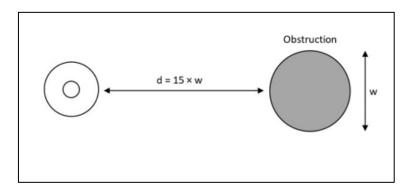
1.1.5 The equipment should be installed and mounted in accordance with the manufacturer's requirements in the technical documentation. If two Iridium antennas are installed, the antennas should be installed such as to ensure electromagnetic compatibility.
